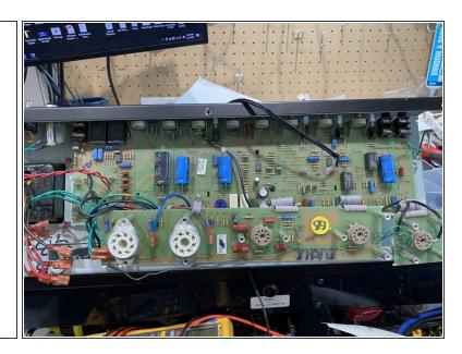
Remove the smaller tube PCB that supports the tube sockets: Remove the tubes and then remove the small black screws that hold both the larger tube PCB and the smaller V1 tube PCB to the chassis. Gently lift both tube PCBs free of the chassis
