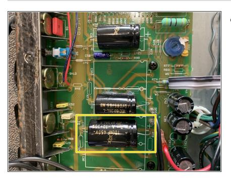
Install the Electrolytic 100uf/ 450V cap at C31
