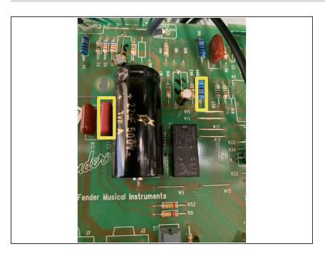
Install 1/2W 56k in R44 and .022uf capacitor in C23
